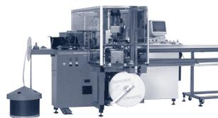
Designed with flexibility and expandability in mind, the Komax 411-S alpha can accommodate up to three processing stations. In the standard version, stations 2 and 3 are equipped with a crimping press. Station 1 can be with a seal applicator. Optional equipment is available for other processes such as tinning, marking, and intermediate stripping. Other features include fast terminal reel exchange, graphic user interface, and good/bad sorting.
