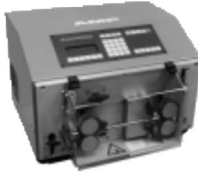
Fully electric, microprocessor-controlled bench machine for processing wire and round and flat cable. Features LED display prompts for easy-to-follow setups and operation, automatic wire loading and unloading, and universal V-type blades. Prefeeder, 1214317-1, and wire stacker, 1214318-1, available for unattended operation. Process 5 200 wires per hour (22 AWG [0.3 mm<sup>2</sup>], 4 [100] length, partial strip
