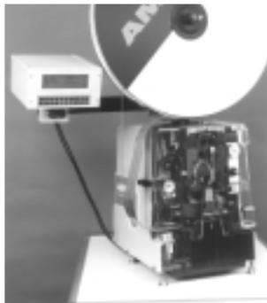
Semiautomatic bench crimping machines that also strip the wire, and are therefore used for terminating jacketed cable. Feature manual precision adjustment of crimp height, keyed strip blades for faster, more accurate setups, and an efficient scrap removal system. All adjustments can be made from the front of the machines without special tools. Available with crimp quality monitoring.
