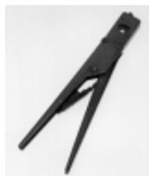
Premium grade hand tools. Feature ratchet control to provide complete crimp cycle. Die sets close in a straight line. Include a contact locator and wire stop, plus an insulation crimp adjustment lever, when applicable. Approximate weight 1.3 lb [0.59 kg]
