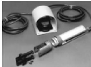
Lightweight, air-operated modular tooling system. Accepts a wide variety of interchangeable heads for crimping various types of contacts, terminals and splices onto wires ranging 6-26 AWG [13-0.12 mm<sup>2</sup>], plus coaxial and fiber optic cable. Available with either hand- or foot-actuation switch. Optional ratchet control available to provide complete crimp cycle.
