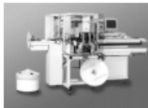
This fully-automatic, PC-controlled leadmaker can be equipped with up to three processing stations enabling the crimping of both ends of the wire, double-crimp connections with three different contacts, single-ended seal applications, tinning or ink-jet marking. Features include ultra-short conversion times, easy-to-use graphic-based TopWin interface with multiple-language capability, crimp force analyzer with statistical analysis, seal monitoring, and integrated
