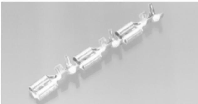
Receptacle contacts are manufactured from 0.32 [.013] thick material. Uncrimped contact length is approximately 19.7 [0.776] not including the cut-off tab.
