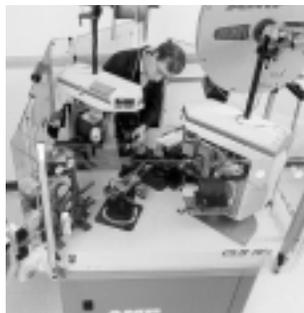
Fully-automatic machines that measure, cut, strip and terminate single leads. Microprocessor-controlled, and programmed and operated using an easy-to-follow, menu-driven touchscreen. Features include direct-drive terminating units with precision crimp height adjustment, fully programmable setups, wire runout and splice detection, and motorized pre-feed with wire straightener. Crimp quality monitoring is also available.
