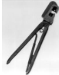
Premium grade hand tool. Features ratchet control to provide complete crimp cycle. The interchangeable die sets close in a straight line to minimize contact or terminal rotation during crimping. When applicable, user-assist features, such as a contact or terminal locator and a wire stop, are built into the die set. Approximate weight 1.9 lb [0.86 kg].
