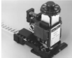
Interchangeable applicators for crimping products reeled side-by-side on single or dual carrier strips (primarily closed-barrel terminals and open-barrel contacts). Similar design as the end-feed version. All side-feed applicators include a wire stop to help correctly position the wire end in the crimping target area.
